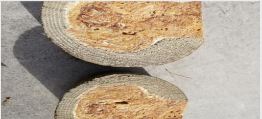
Polywater UPR expanded into the walls of the cavity created by the woodpecker and successfully filled the void.
